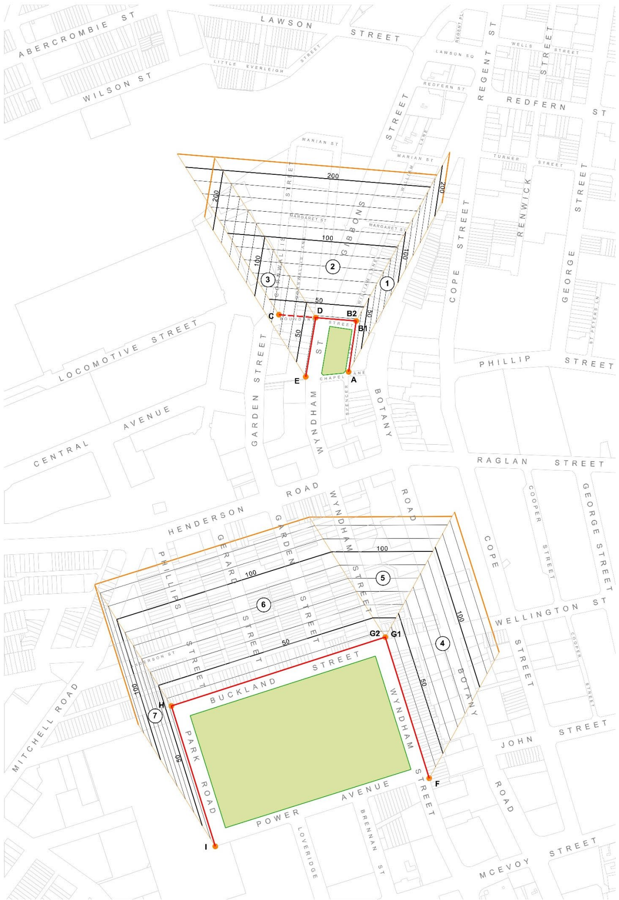
Figure 46. Map showing solar access planes to protect Daniel Dawson Reserve and Alexandria Park
